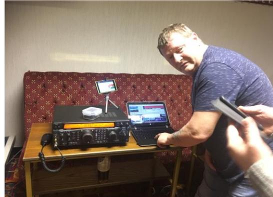
Tom M0HYE brought in his portable DMR hotspot, it has a modem which uses a mobile phone network, which is connected to his Shark RF Hotspot which enables him to use his DMR handheld to talk to the world whilst mobile or portable, a very neat little setup,
